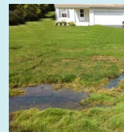
Right: HSTS showing illicit discharge.
