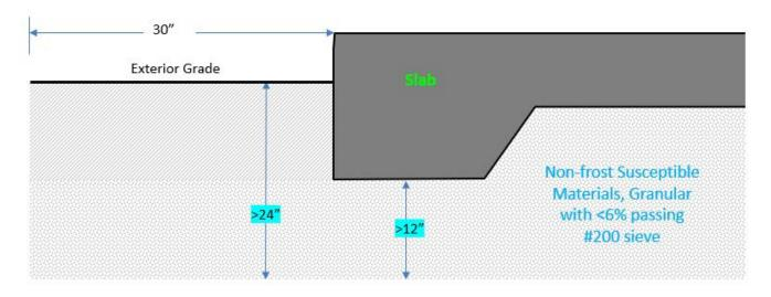
For subgrade prepared as recommended and properly compacted fill, a modulus of subgrade reaction, *k* value, of 50 pounds per cubic inch (pci) may be used in the grade slab design based on correlation to values typically resulting from a 12-inch diameter plate load test. However, depending on how the slab load is applied, the value will have to be geometrically modified. The value should be adjusted for larger areas using the following expression for cohesive and cohesionless soil:
