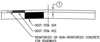
$\bigcirc$  ROADWAY AND COMMERCIAL DRIVES - 8" THICK CONCRETE RESIDENTIAL DRIVE - 6" THICK CONCRETE
